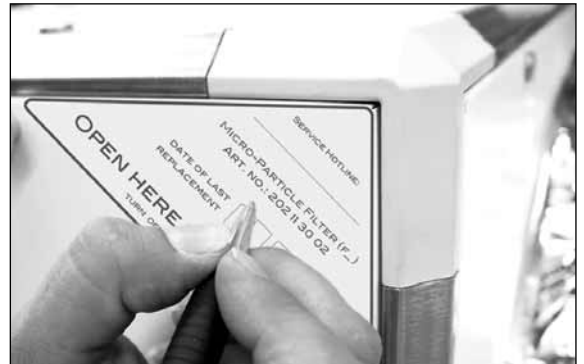
8. Fill out the filter replacement label with scheduled date of next filter replacement. This should be no more than 3 years from current date, and affix on outer panel.
