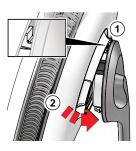
Tilt and hook the air purifier onto the stand head and snap together.
