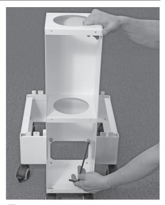
Remove the cover from the support column by unscrewing the six M4 screws. Then fit the support column to the base platform with the four M8 screws and double set of washers.
