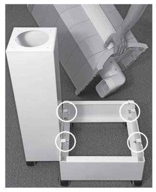
Remove the 4 butterfly screws and washers from the base platform. Carefully lift the IQAir device onto the base platform with the opening of the suction adapter duct facing the support column.
