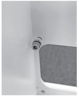
The plastic washers should be positioned after the metal washers to prevent damage to the powder coating of the support column. Securely tighten all screws.
