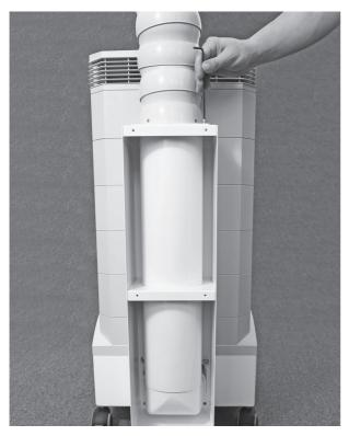
Secure the duct in place using the four M4 screws and plastic washers.
