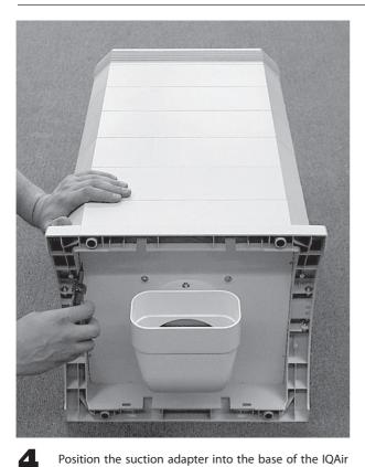
Position the suction adapter into the base of the IQAir device. Use the supplied Torx screwdriver to secure the adapter with the eight T8 screws. All screws must be equally tight to provide a good seal, but be careful not to over-tighten the screws.
