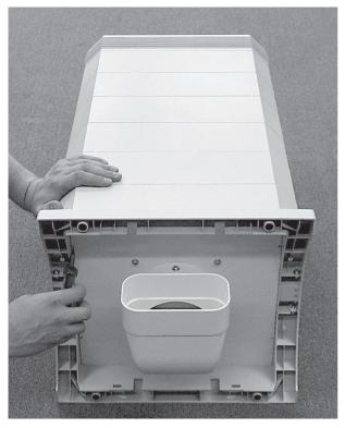
Position the suction adapter into the base of the IQAir device. Use the supplied Torx screwdriver to secure the adapter with the eight T8 screws. All screws must be equally tight to provide a good seal, but be careful not to over-tighten the screws.
